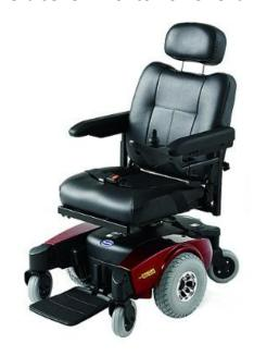
The Pronto power chair is a mid wheel drive chair with a range of adjustments available. On board are 2x 32Ah AGM dry cell batteries which can give a max speed of 6kmh(3.8mph) and a max range of 19km(11.8miles), although the range and speed of the chair may vary depending on the weight of the user, terrain type, outside temperature and battery charge.
